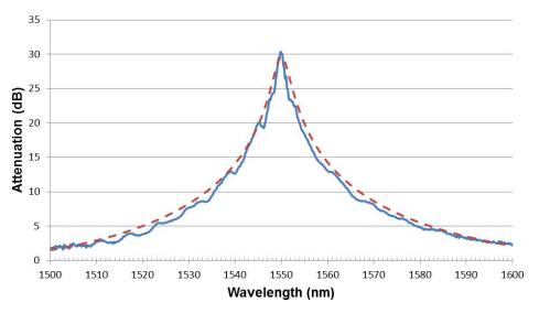
Wavelength response of  $LP_{01}$  transmission for mechanical LPG. Solid curve shows experimental results and dashed curve theoretical curve with the same number of coupling points and coupling coefficient.
