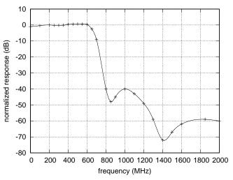
Test conditions: Light input 100  $\mu\mathrm{W}$  at 1550 nm, modulated via EOM.
